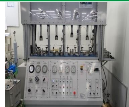
High Pressure Gas Tester (Water)
