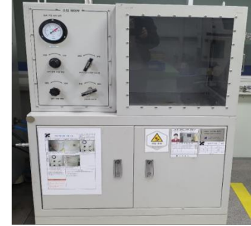
Pressure Test Unit (Water)
