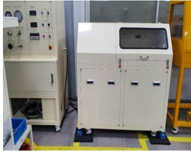
Rotary Flex Tester (with Strain Gauge)
