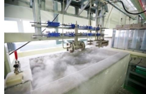
Cryogenic Valve Tester (2 Boosters and 9 Chambers)
